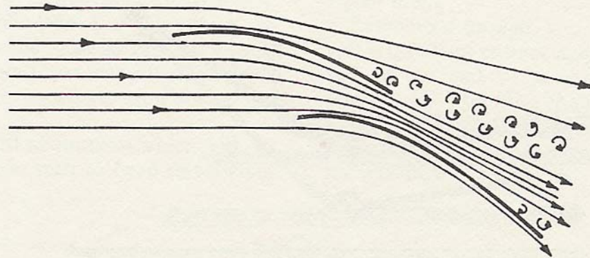
Figure 2B: Both headsail and mainsail should be parallel at exit so wind can pass through with minimum disturbance
