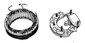
(7) Separate the diode assembly and the brush regulator assembly by removing the 3mm dia rivet which connects these two parts and then unsolder the L terminal connection.
