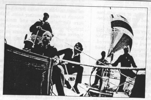
Steering downwind requires constant communication between helmsman and spinnaker trimmer. The trimmer must think of himself as an extension of the driver's sense of feel.
